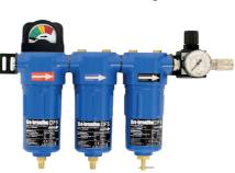
The e-breathe compressed air filter station has been designed for the preparation of technical compressed air. The high performance filters included in the respective stations capture and remove solid particles, aerosols, oil vapours and odours from the compressed air flowing through. Depending on the application, a 2-stage or 3-stage filter system can be used.
