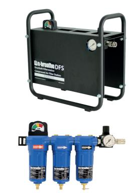
The e-breathe compressed air filter station has been designed for the preparation of technical compressed air. The high performance filters included in the respective stations capture and remove solid particles, aerosols, oil vapours and odours from the compressed air flowing through. Depending on the application, a 2-stage or 3-stage filter system can be used.
